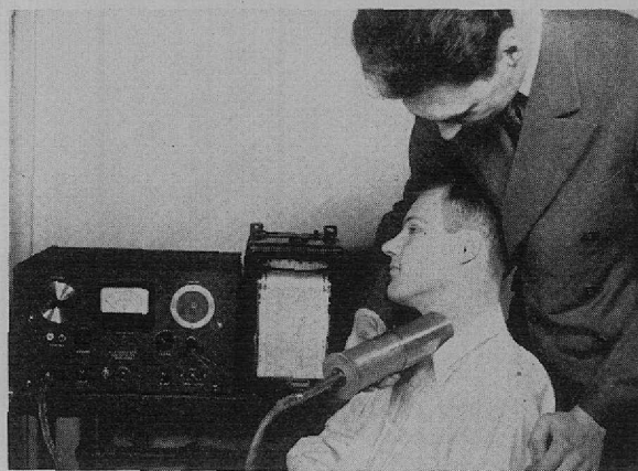
FIGURE 184. USE OF COUNTING RATE METER FOR DETERMINATION OF RADIOACTIVE IODINE IN THYROID OF A PATIENT
