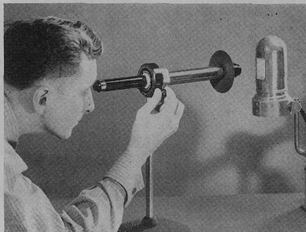
FIGURE 144. POLARIMETER UTILIZING POLAROID FILM
