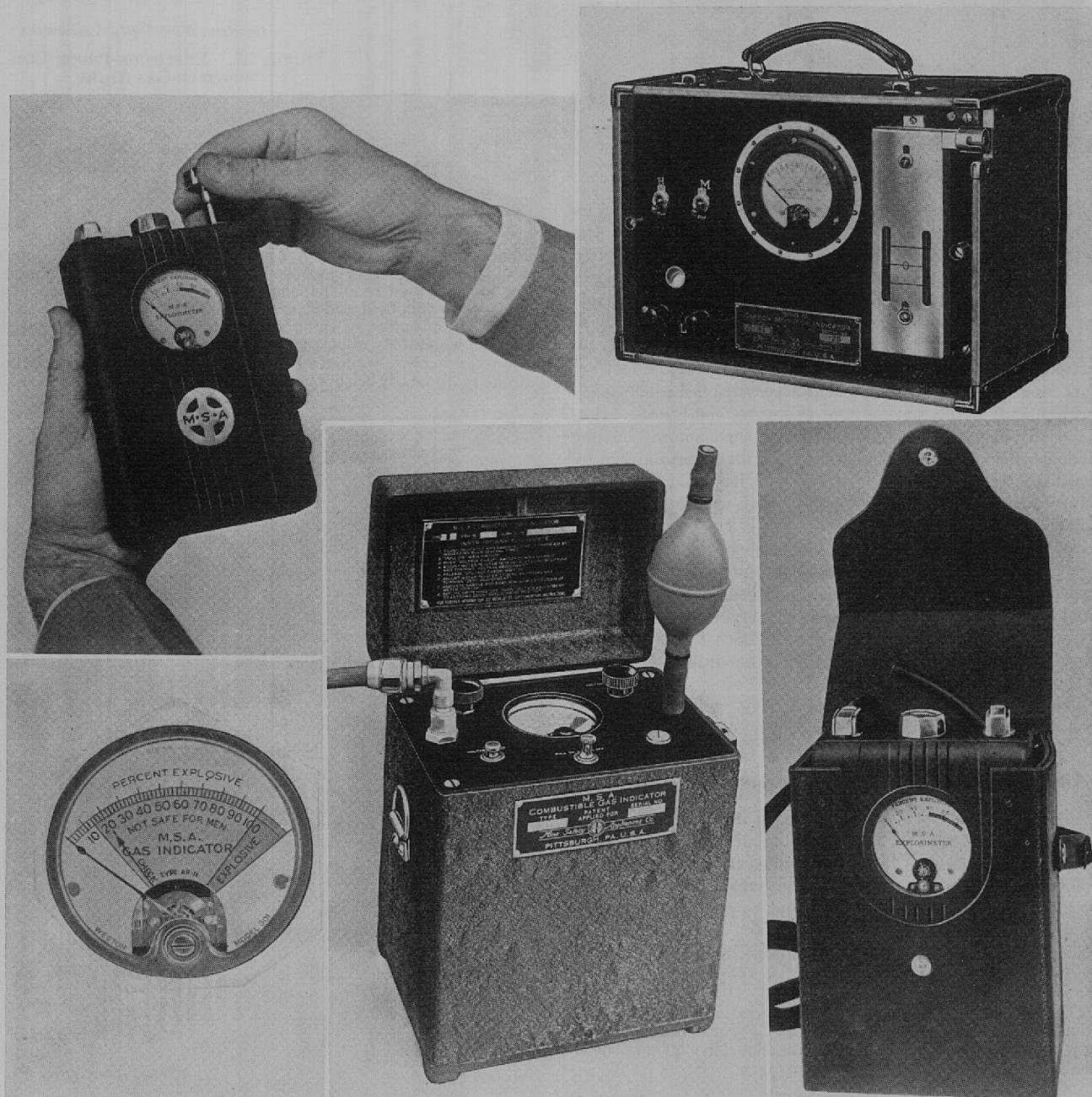
FIGURE 35. (Upper Left and Lower Right) EXPLOSIMETER. (Center) COMBUSTIBLE GAS INDICATOR. (Lower Left) GAS INDICATOR. (Upper Right) CARBON MONOXIDE INDICATOR
