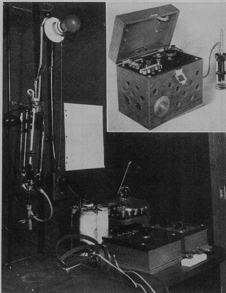
FIGURE 159. ELECTRICAL CONDUCTIVITY APPARATUS FOR SUGAR ASH DETERMINATIONS IN A CONSTANT-TEMPERATURE ROOM (20° C.) (Upper Right) SUGAR ASH BRIDGE. Courtesy Leeds & Northrup Co.
