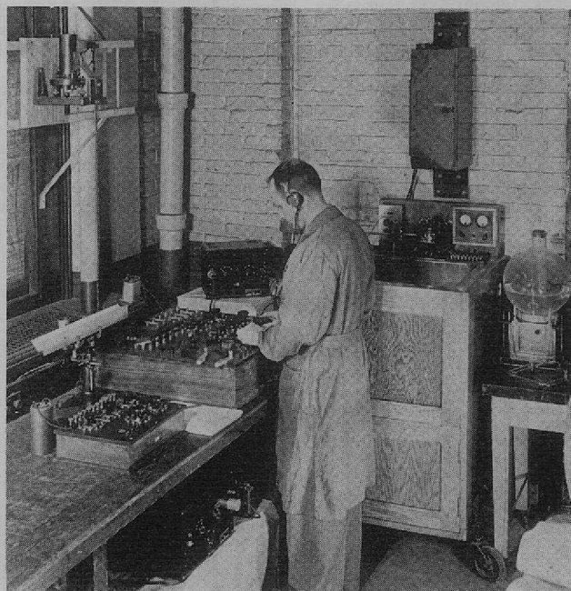
FIGURE 156. HIGH-PRECISION CONDUCTANCE ASSEMBLY Jones bridge, vacuum tube oscillator, output amplifier, Mueller bridge for temperature measurements, and thermostat regulating to \pm 0.001^\circ \text{C} .
